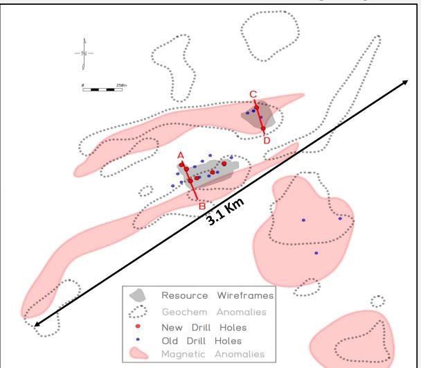
Two mineralised zones drilled by PNL (Sections A-B and C-D); geologically similar & 600m apart
